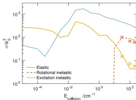
FIG. 3. Integral scattering cross sections for elastic, rotationally inelastic, and excitation inelastic transitions. Lines correspond to results of coupled-channels calculations, where symbols refer to approximate semiclassical calculations.
